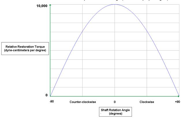
Note that we can modify the amount of restoration torque produced by the magnetic spring return and thus, actuators can be manufactured which produce the same torque, but have reduced magnetic spring return action. Such actuators will provide a greater amount or rotation with less input electrical current. This may be desirable in low power applications. Likewise, magnetic spring return can be increased as well.
