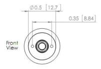
Front screw holes: #0-80 thread Front shaft diameter: 0.118 [3.00]
