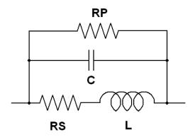
RS is the series resistance of the copper coils
