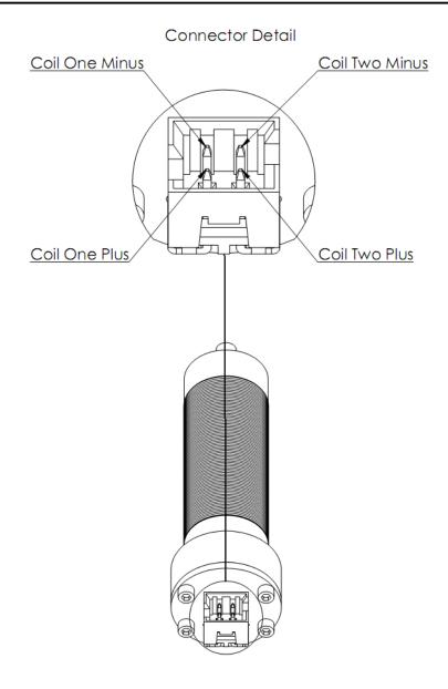
Actuator mating connector is 4-pin Molex part number 51110-0460
