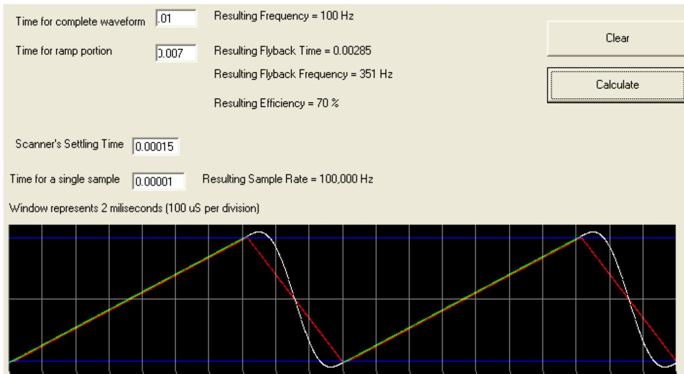
The Mach-DSP servo driver has accompanying Application Software that runs on a Windows-based PC. The software is capable of monitoring all parameters of the scanner during operation. The software also includes a built-in oscilloscope function. This comes in handy as it can be used to measure virtually any quantity of the overall scanning system.
