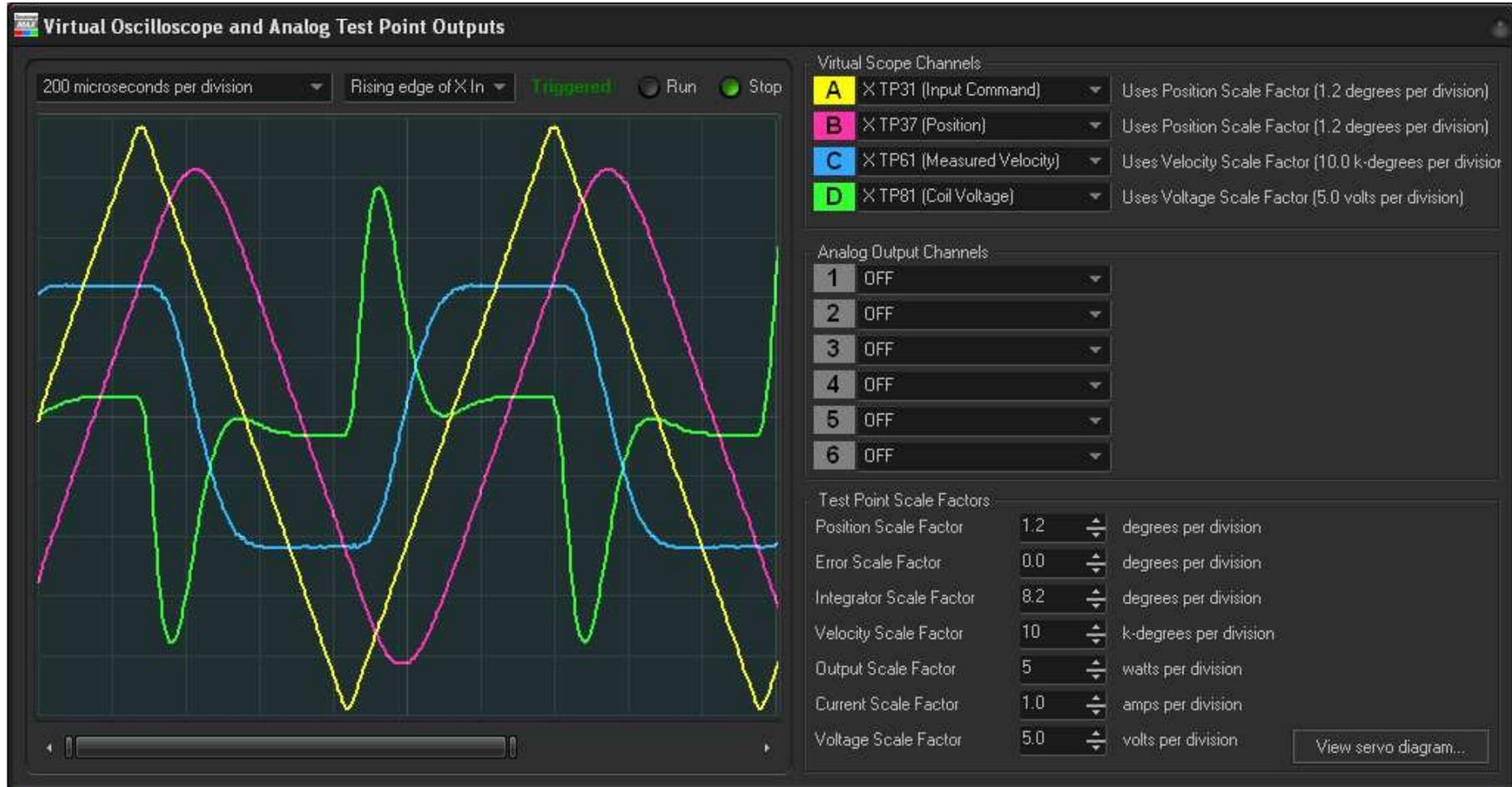
Reducing the scan amplitude to 20-degrees peak-to-peak (around 24-degrees of command) or below, allows the original 2.5kHz servo gains to be used. This amplitude is about the maximum for a frequency of 1kHz, to retain a good looking triangle wave with decent periods of time with constant velocity scanning. The relevant data-points are expressed in the partial table below.
