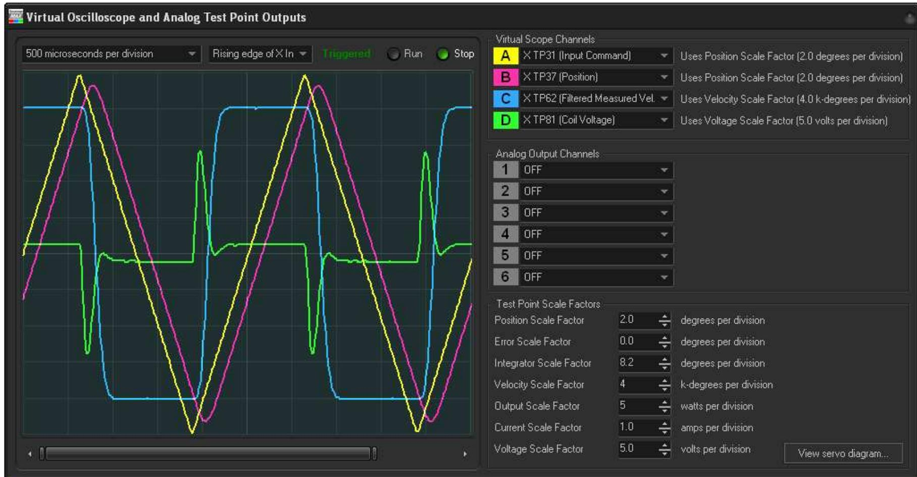
The Blue trace shows scanning velocity. For imaging applications, it is most desirable that this be “flat” on the top and bottom, representing periods of constant velocity. Here at 400Hz we have a nice flat velocity, with not too much time taken for the turn-around at each corner of the triangle-wave. Here we can see that the command is 40-degrees, but the scan is only 37 degrees.
