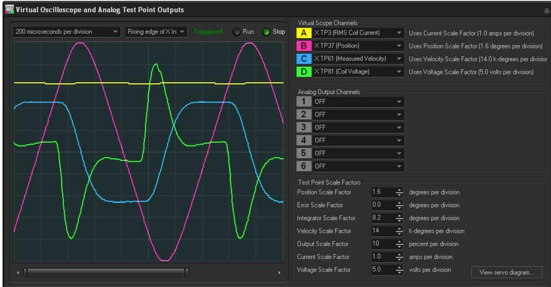
As mentioned in the introduction to the section on triangle-wave scanning, in order to prevent the coil voltage from exceeding +/- 20V, servo gains had to be reduced for frequencies of 700Hz or greater. Alternatively, cycloid waveforms (triangle-waves with rounded tops and bottoms on the command) could have been used.
