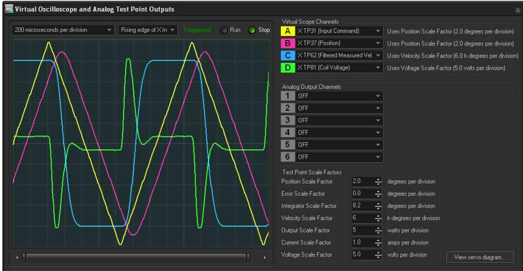
The Blue trace shows scanning velocity. Here the triangle-wave scan still shows nice flat velocity, with not too much time taken for the turn-around at each corner of the triangle-wave.
