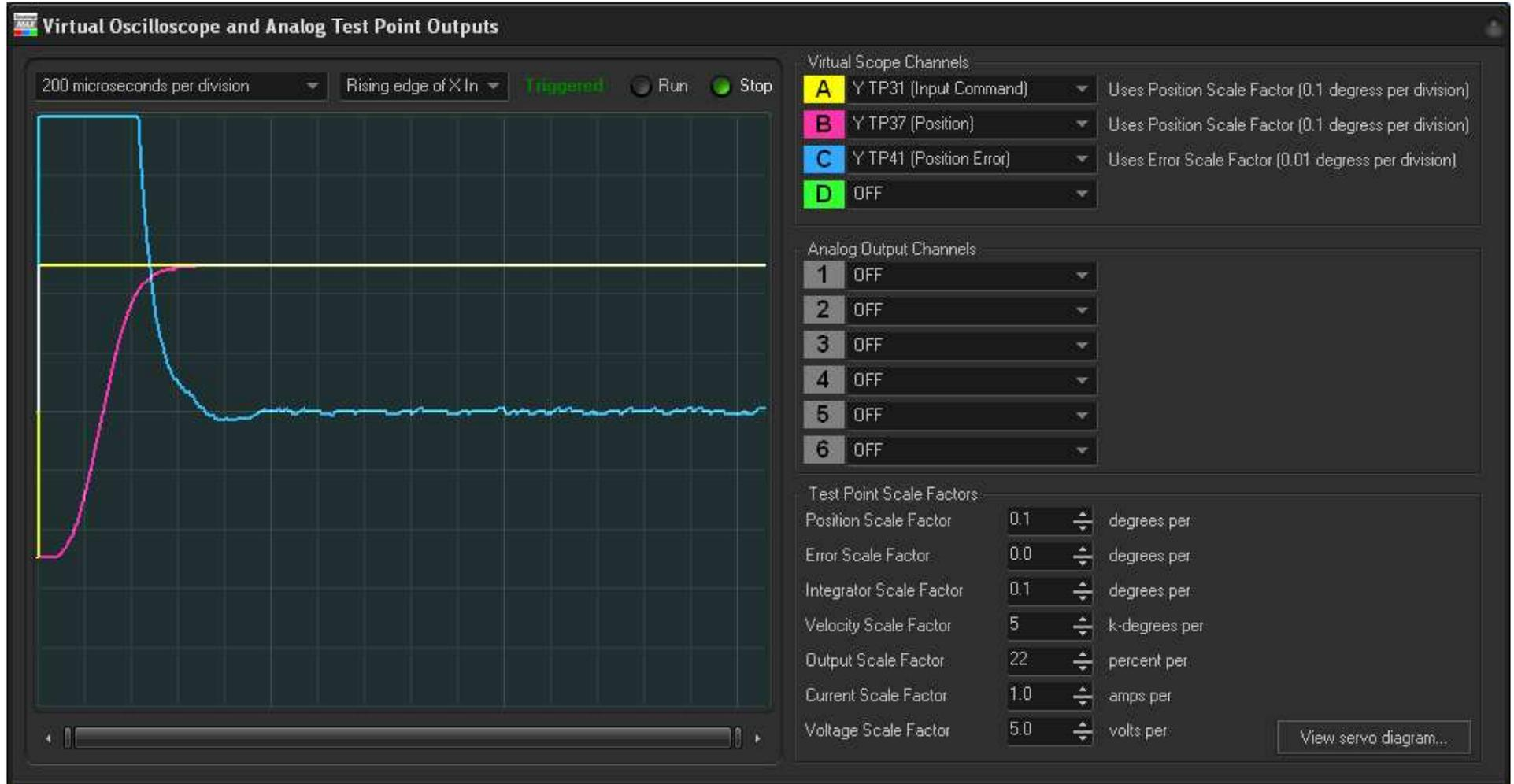
Position is settled to within  $1/100^{\text{th}}$  of 1 mechanical degree (0.01 degrees) within 550 microseconds. Since the step is 0.5 mechanical degrees, 0.01 degrees represents 2% of the 0.5 degrees, or 98% of the full step.
