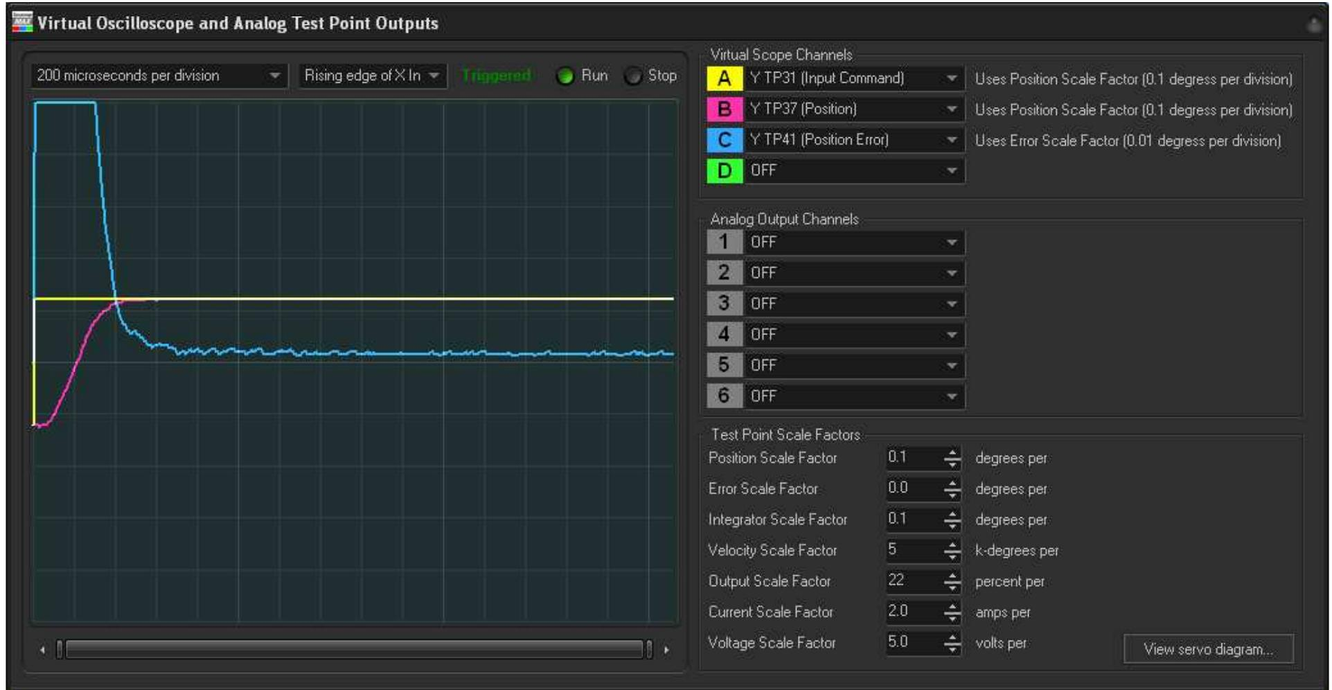
Position is settled to within  $1/100^{\text{th}}$  of 1 mechanical degree (0.01 degrees) within 400 microseconds. Since the step is 0.25 mechanical degrees, 0.01 degrees represents 4% of the 0.25 degrees, or 96% of the full step.
