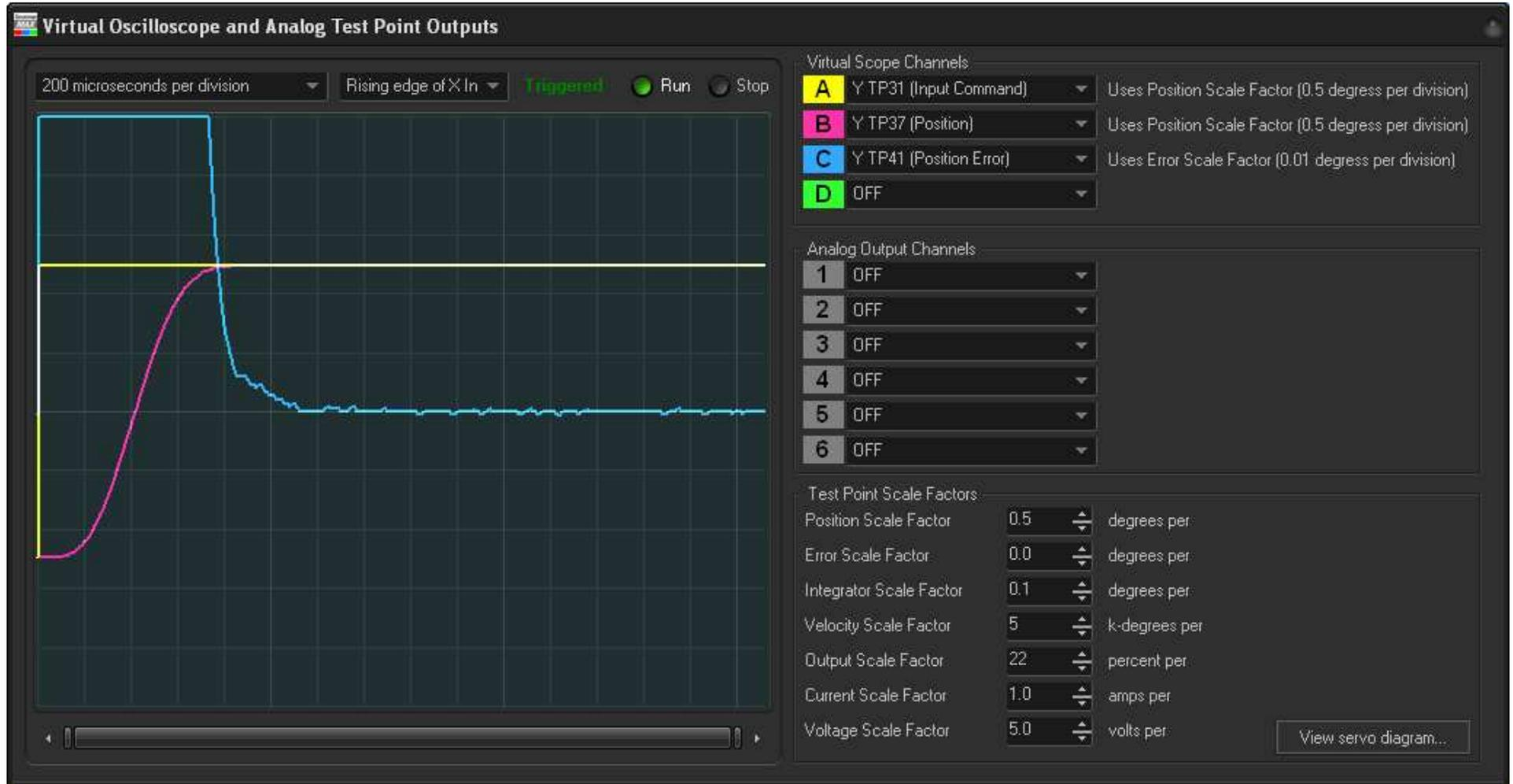
Position is settled to within  $1/100^{\text{th}}$  of 1 mechanical degree (0.01 degrees) within 825 microseconds. Since the step is 2.5 mechanical degrees, 0.01 degrees represents 0.4% of the 2.5 degrees, or 99.6% of the full step.
