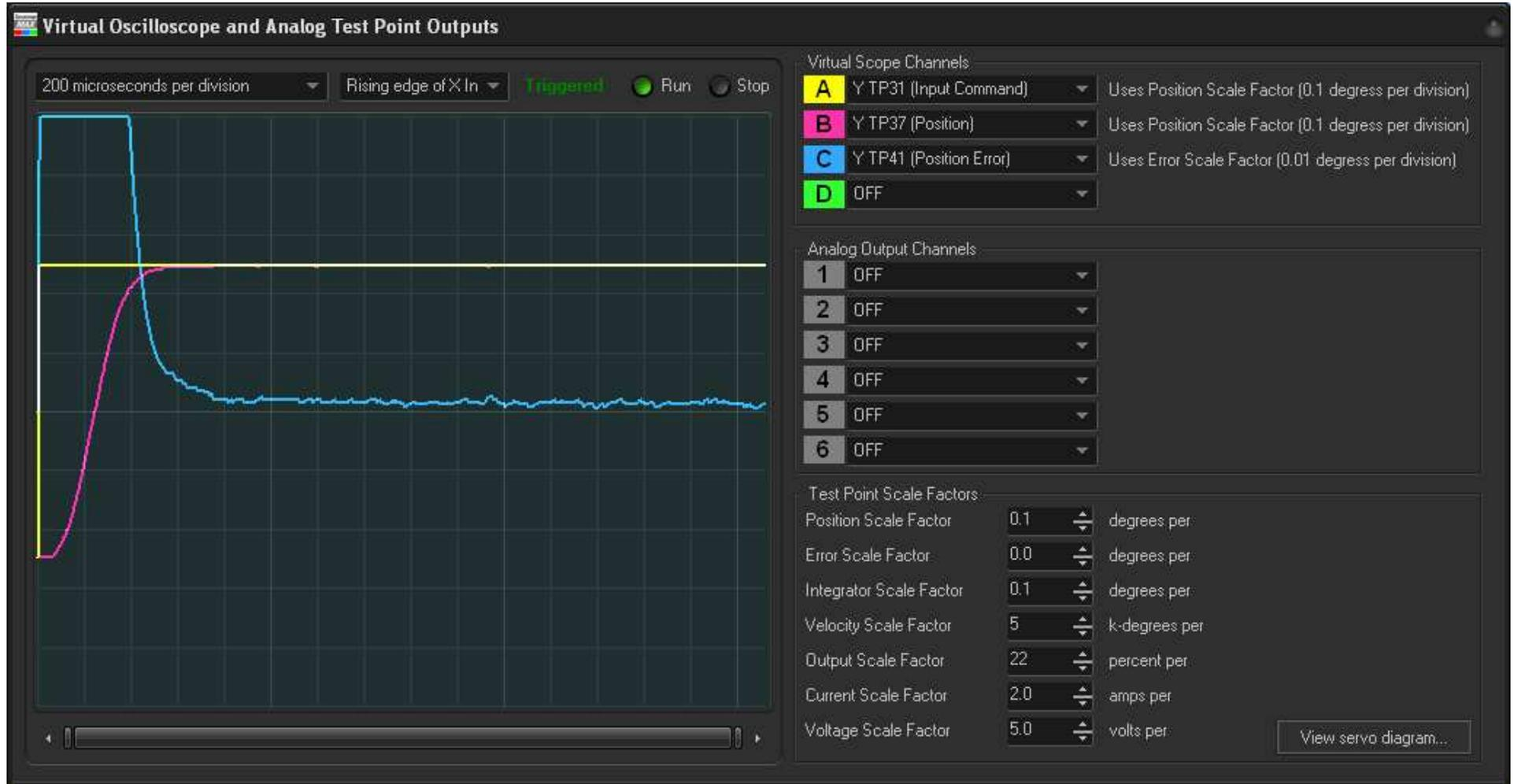
Position is settled to within  $1/100^{\text{th}}$  of 1 mechanical degree (0.01 degrees) within 500 microseconds. Since the step is 0.5 mechanical degrees, 0.01 degrees represents 2% of the 0.5 degrees, or 98% of the full step.
