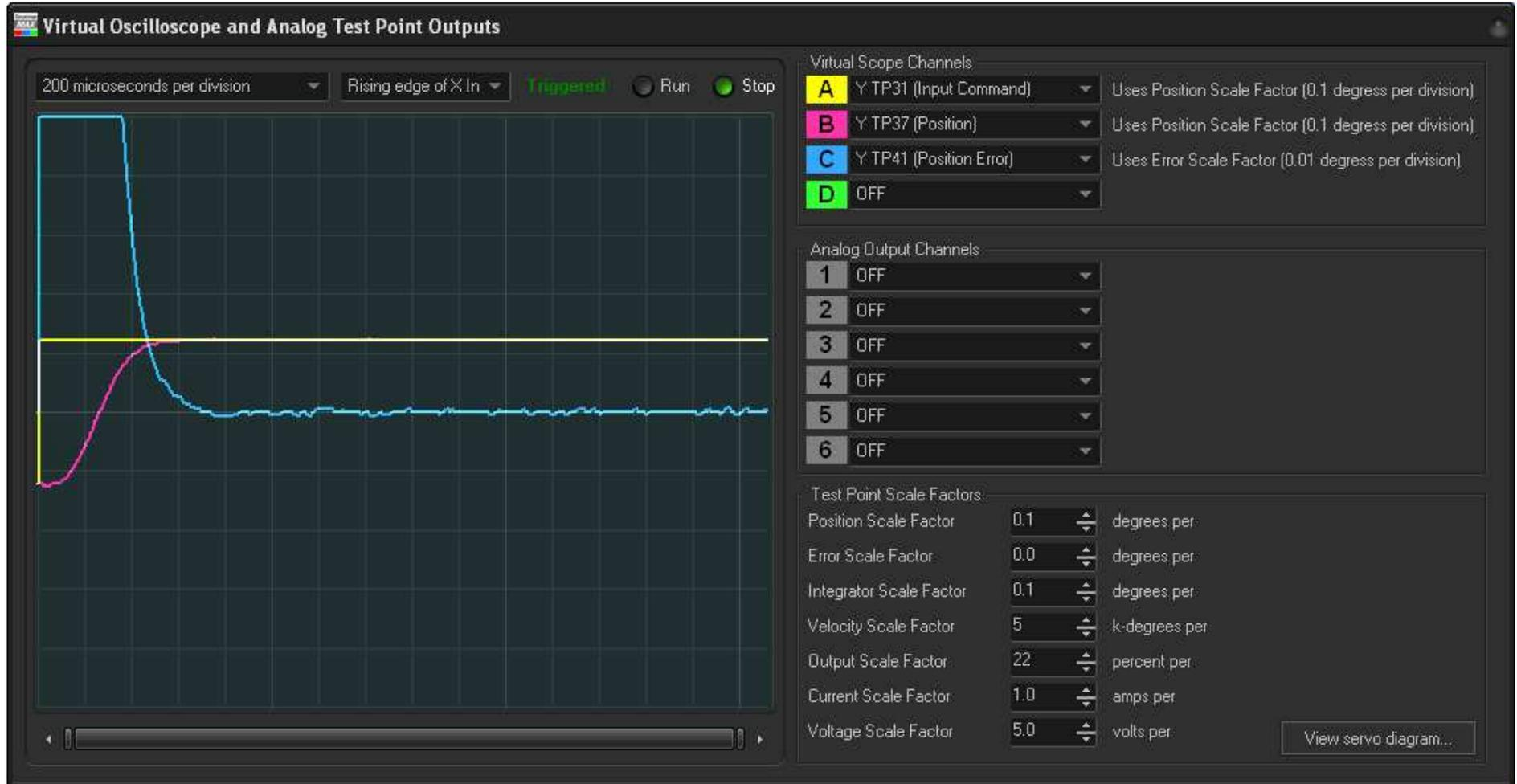
Position is settled to within  $1/100^{\text{th}}$  of 1 mechanical degree (0.01 degrees) within 500 microseconds. Since the step is 0.25 mechanical degrees, 0.01 degrees represents 4% of the 0.25 degrees, or 96% of the full step.
