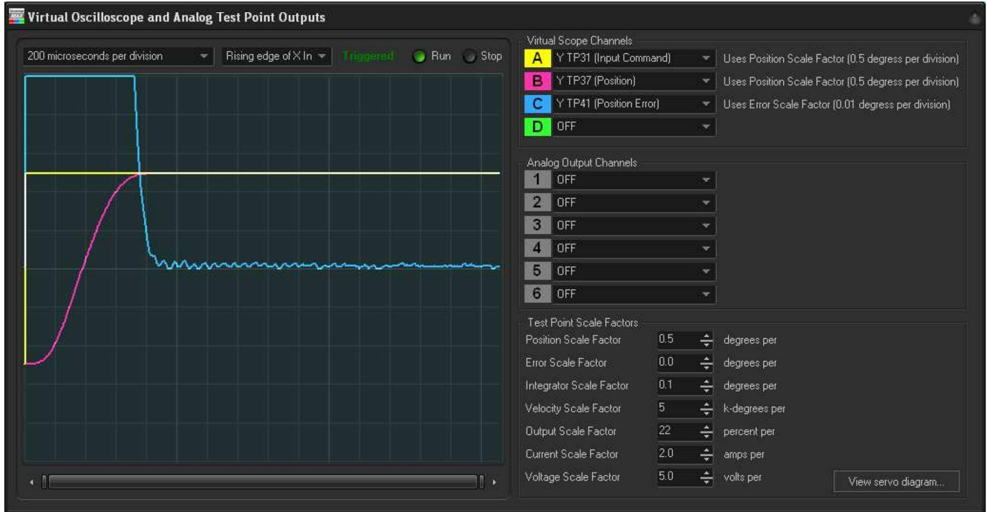
Position is settled to within  $1/100^{\text{th}}$  of 1 mechanical degree (0.01 degrees) within 800 microseconds. Since the step is 2.5 mechanical degrees, 0.01 degrees represents 0.4% of the 2.5 degrees, or 99.6% of the full step.
