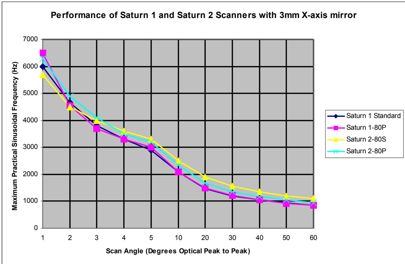
Although the difference is subtle, it is apparent that the combination of the Mach-DSP servo driver and Saturn 2B-80S offers the highest performance for frequencies up to 3600Hz. At higher frequencies, the impedance caused by inductance would require a higher drive voltage to drive this scanner to its maximum potential. The Mach-DSP can only practically deliver up to 52V peak-to-peak with +/-30V power supplies, so this presents the limiting factor.
