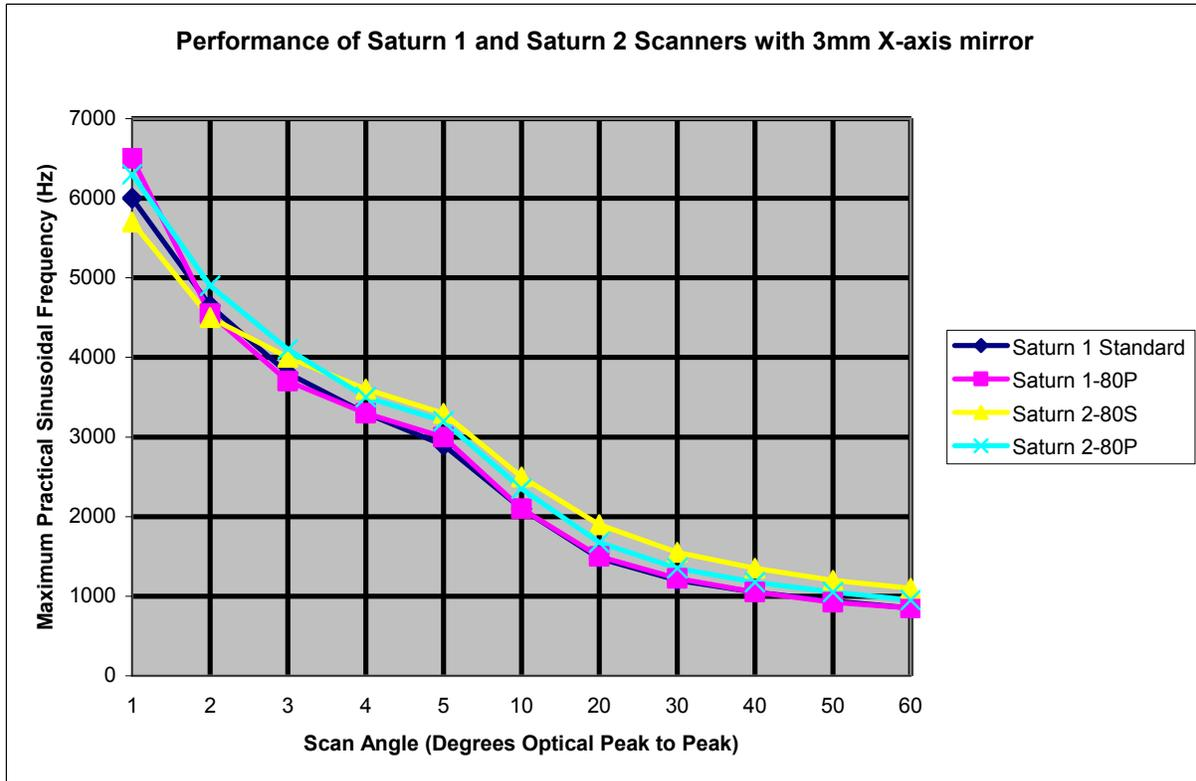
The graph above denotes the actual, tested performance of our Mach-DSP servo driver, driving four separate ScannerMAX scanners, each having our 60-degree, 3mm-aperture X-axis mirror. The scanners tested were the Saturn 1 with Standard coil configuration, Saturn 1 with 80-P coil configuration, Saturn 2 with 80-S coil configuration, and Saturn 2 with 80-P coil configuration.
