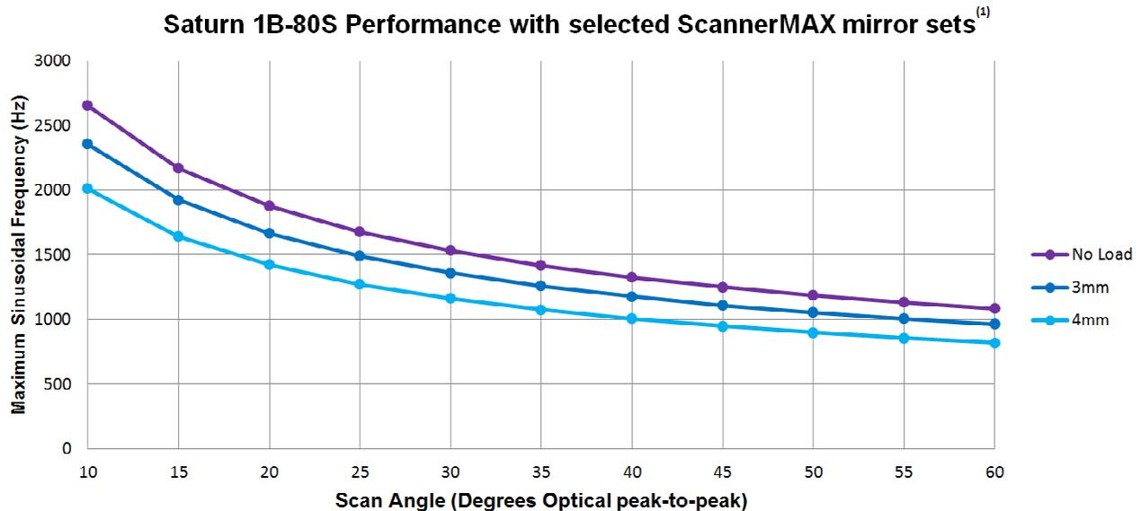
This graph conveys that for a Saturn 1B-80S, with a mirror that can reflect a 3mm beam, it is possible to scan 1000Hz at 55-degree optical peak-to-peak.
