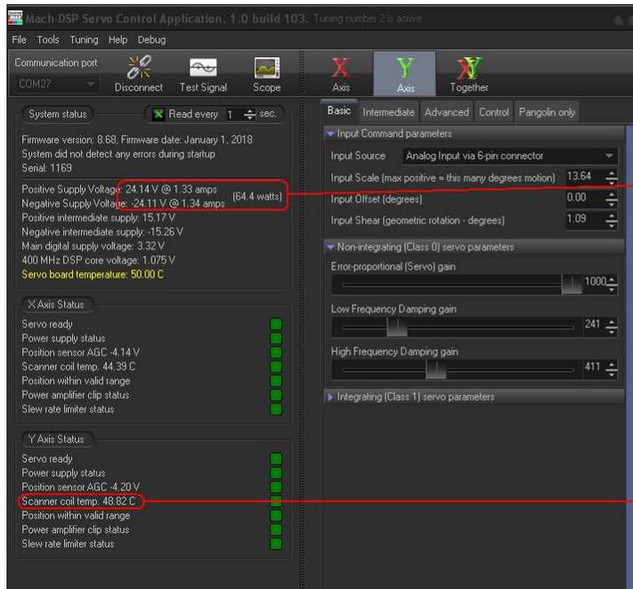
Using our Standard Saturn this pattern requires +/-24V power supplies and a bit more than 1.3 amps per rail.
