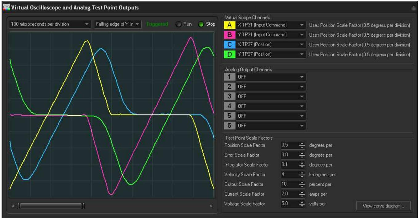
It can be seen that the X and Y input command waveforms (yellow and pink traces) are larger in amplitude than the X and Y position waveforms (blue and green traces). This is because the servo system acts as a low-pass filter (5kHz low-pass with this particular tuning). This also essentially means that the resulting position waveforms are “rounded” when compared the command waveforms.
