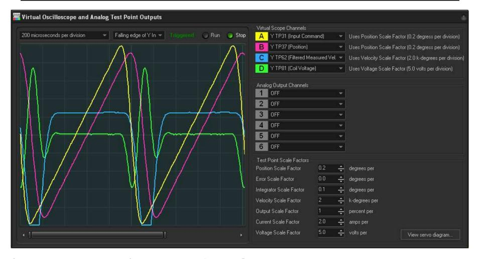
Cycloid retrace program was set for 760 microsecond "ramp time", and a corresponding 240 microsecond retrace time.
