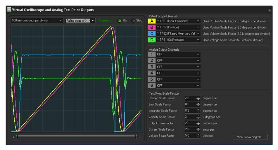
Cycloid retrace program was set for 4.33 millisecond "ramp time", and a corresponding 670 microsecond retrace time.
