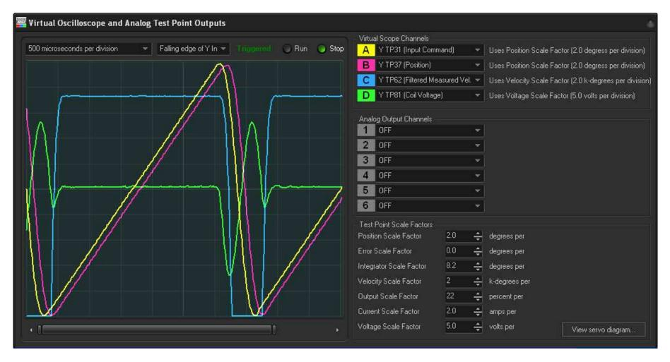
Cycloid retrace program was set for 2.6 millisecond "ramp time", and a corresponding 733 microsecond retrace time.
