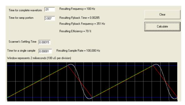
The Mach-DSP servo driver has accompanying Application Software that runs on a Windows-based PC. The software is capable of monitoring all parameters of the scanner during operation. The software also includes a built-in oscilloscope function. This comes in handy as it can be used to measure virtually any quantity of the overall scanning system.
