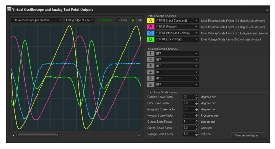
Cycloid retrace program was set for 330 microsecond "ramp time", and a corresponding 170 microsecond retrace time.
