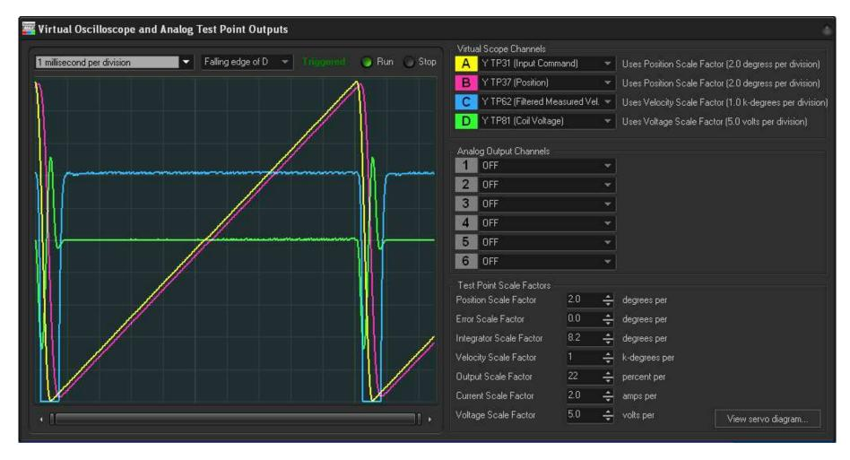
Cycloid retrace program was set for 9.35 millisecond "ramp time", and a corresponding 650 microsecond retrace time.
