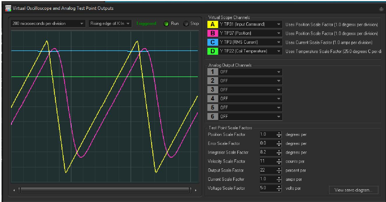
In this case, the coil current is 3.8 amps RMS and coil temperature is around 50 degrees C. The scanner will be dissipating 26 watts, and power required from the power supply is around 2.2 amps per rail.
