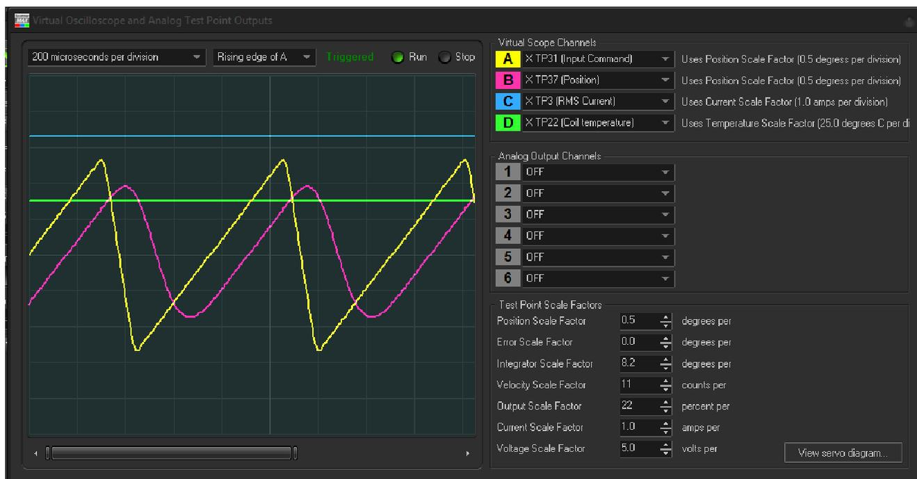
The oscilloscope shows that the RMS current being driven into the scanner is roughly 3.3 amps and coil temperature is only around 35 degrees. Note that at this current, the scanner will be dissipating 13 watts of heat, which is certainly manageable. Power required from the power supply is around 1.9 amps from each of the +24V and -24V supply rails.
