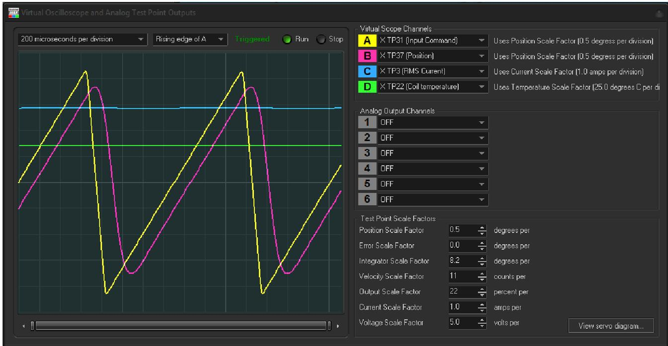
In this case, the coil current is 2.9 amps RMS and coil temperature is around 32 degrees C. The scanner will be dissipating 10 watts, and power required from the power supply is around 1.6 amps per rail.
