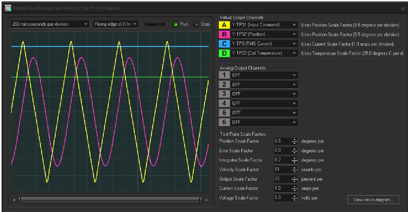
In this case we see that the RMS current being driven into the scanner is around 4.1 amps, and coil temperature is around 55C (assuming the scanner body is 30C). The scanner will be dissipating 30 watts, and power required from the power supply is around 2.25 amps per rail.
