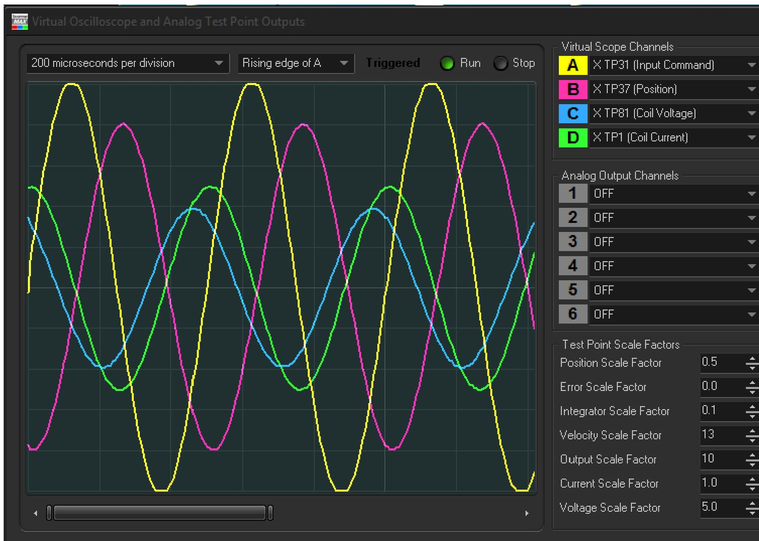
We can see approximately 20 volts peak to peak and 5 amps peak to peak flowing through the scanner coil. RMS Coil current is thus 1.77 amps.
