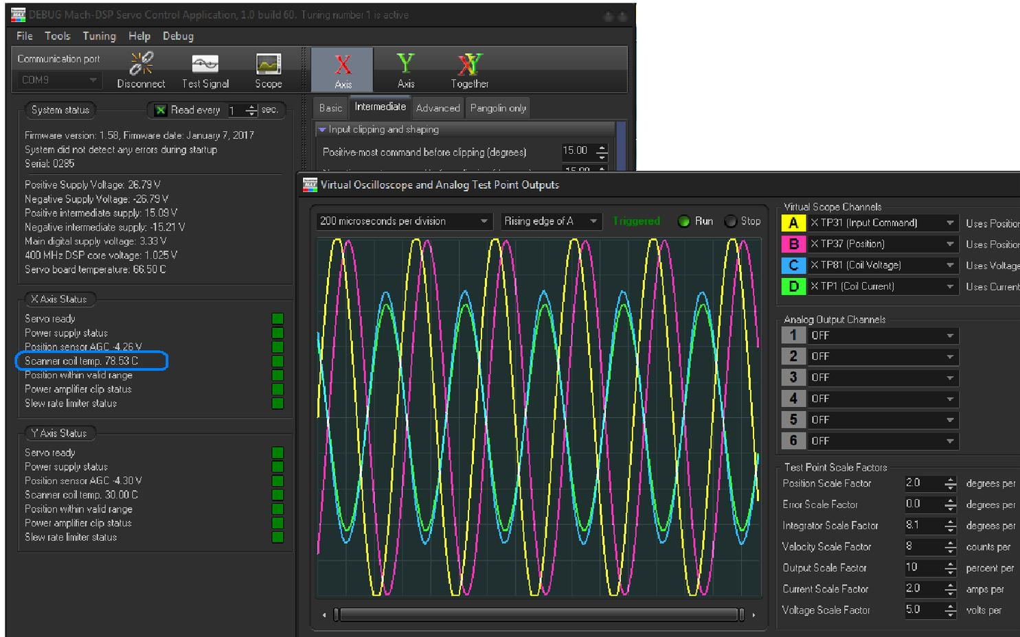
Coil voltage is around 36 volts peak to peak, thus for this frequency, power supplies would need to be at least +/-24V, and +/-30V would be better as a margin for headroom.
