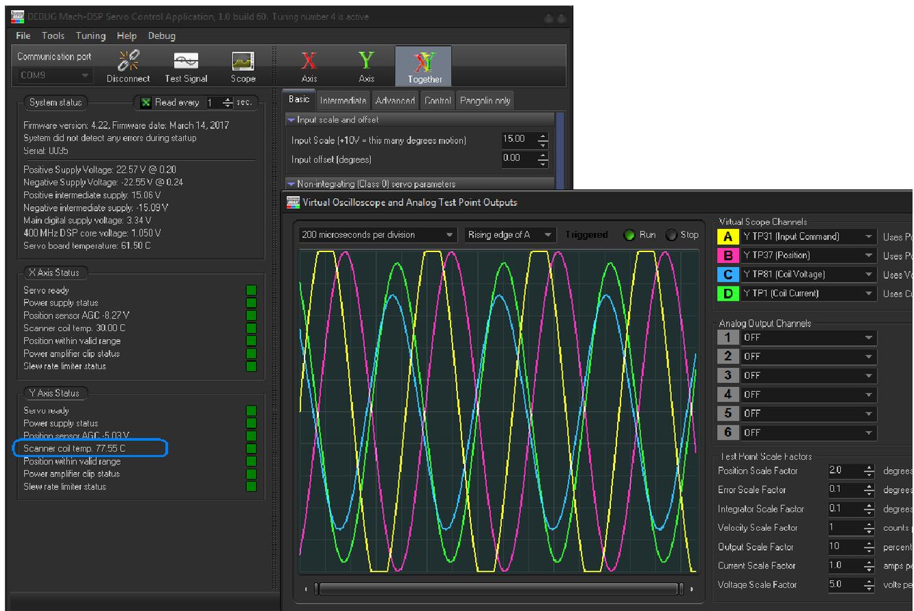
Coil voltage is around 36 volts peak to peak, thus for this frequency, power supplies would need to be +/-24V, with higher power supply voltages providing a margin for headroom.
