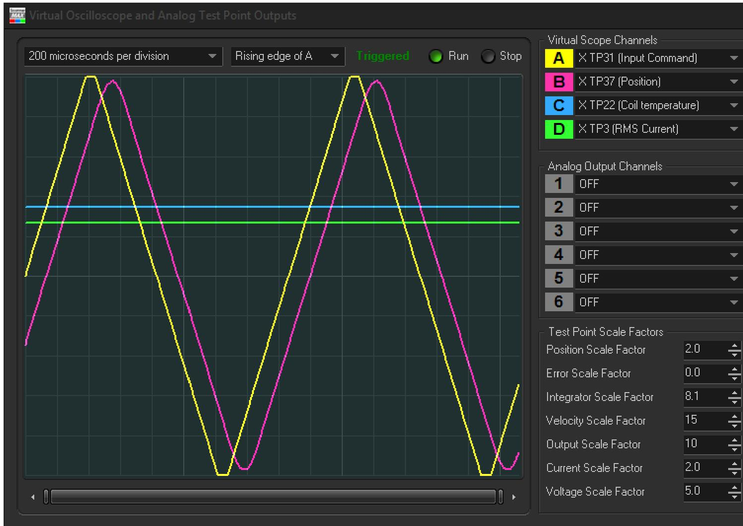
To try to get a sense of the “efficiency” of the triangle wave, I changed the scope channels such that the blue trace shows velocity and green trace shows the actual coil current.
