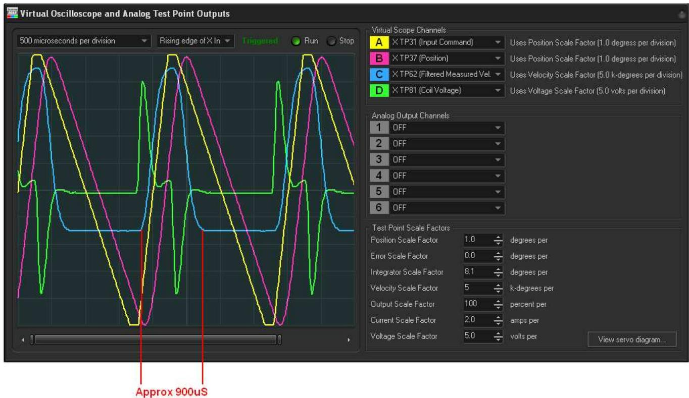
The blue trace of the oscilloscope shows the velocity of the scanner. When the velocity is “flat” (non-changing), this demonstrates that the mirror is traveling at a constant speed, which is highly desirable for imaging applications. During retrace, the mirror speed reaches 22,500 degrees per second, which is equivalent to 393 radians per second.
